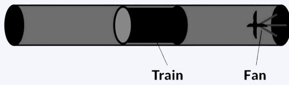
At one end of the railway was a fan which would either suck air out of the tunnel or blow air into it. The train formed an airtight seal with the tube so when the fan started blowing air into the tube, the pressure would build up behind it until it moved away from the fan. When the fan was sucking the air out of the tunnel, this would form a vacuum behind the train, drawing it towards the fan.
