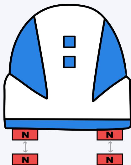
However, some railways use both repulsion and attraction, which is the system used on the Japanese LO Series maglev train. Each side wall has both north and south magnetic poles on them, with one magnet attracting the train's magnet and one repelling the magnet on the train, which balances the two out. This causes the train to levitate.
